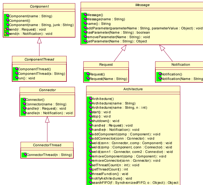
Figure 2. UML class diagram of the framework API.
